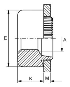
Female thread A = M5Height K = 4.0Outer diameter E = 9.0Plate thickness = 2.9 to 3.1
